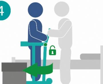
The assistant unlocks and rotates the turntable smoothly left or right to engage the brake rod into one of the five locking positions.
